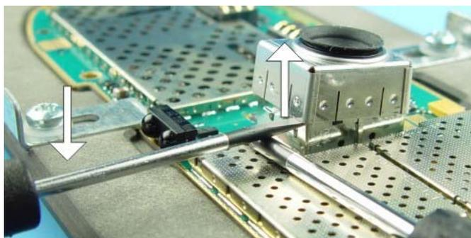
The Camera Module is attached with four snaps onto the Camera Connector. Place the SRT-7 as shown and carefully move the snaps.
