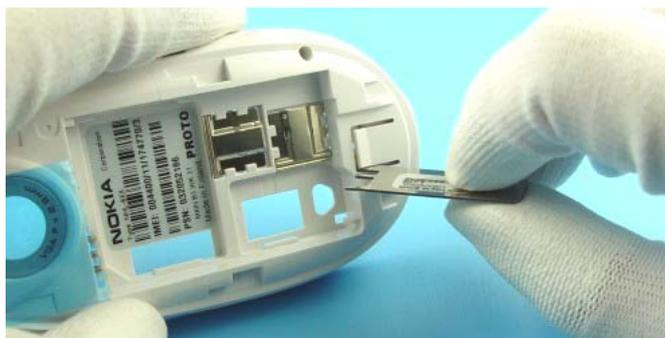
Turn B-Cover to let System Connector with Connector Retainer drop out.
