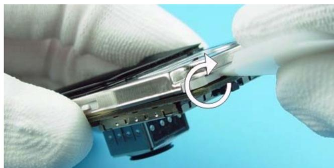
Separate LCD Module from Radio Module.
