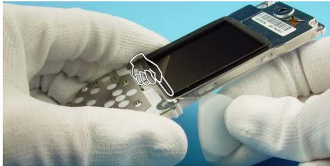
Remove the Shield and Gasket.
