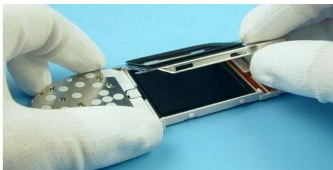
Always protect LCD with protection foil to avoid dust and scratches.
