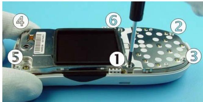
Remove the engine from the B-Cover as shown.
