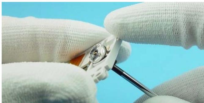
Antenna drops out when turning B-Cover.
