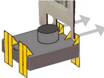
The Camera Module comes up automatically when the snaps are released.
