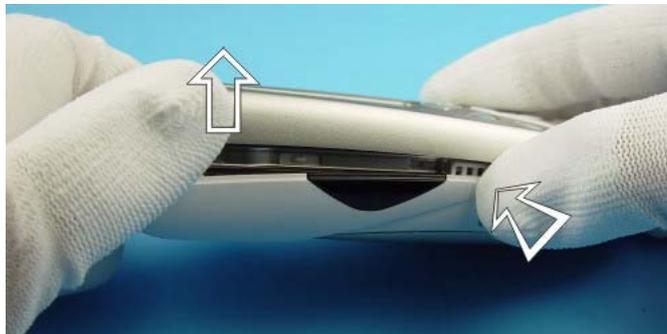
Press the release button (1) before removing the C-Cover.
