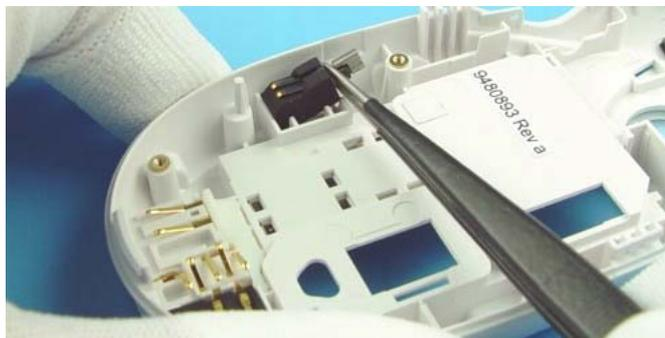
Move SRT-4 through this gap of B-Cover to remove Connector Retainer.
