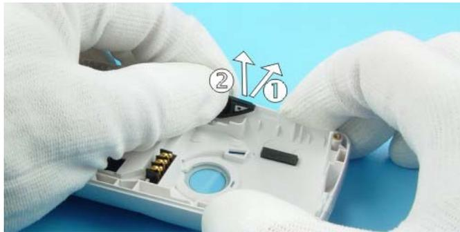
Remove Vibra Motor from its guidance.
