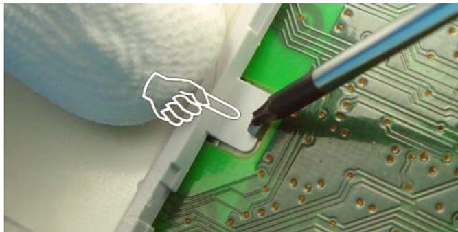
Attach the PWB Insulator and take care of the markings.
