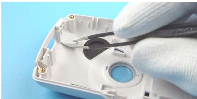
Remove Camera Shield if contacts require cleaning or to change Camera Module.
