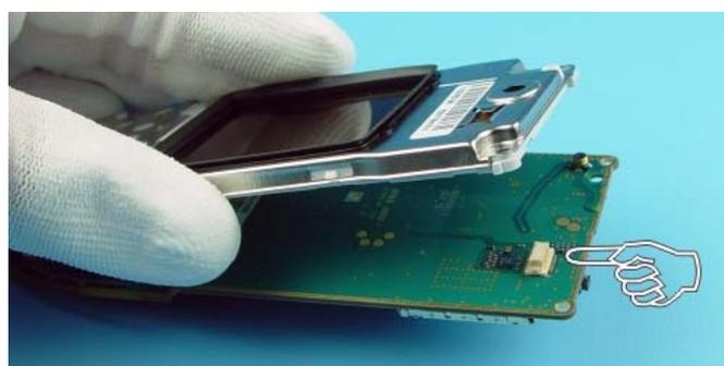
Open the shield snaps using the SRT-6 both sides.
