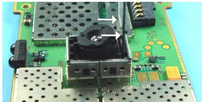
Remove the Camera Module carefully. Note the guide pin when re-assembling.
