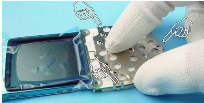
Bend UI Metal Shield latch on backside.
