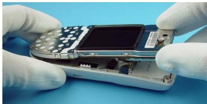
Use the SRT-6 tool to open the connector carefully.
